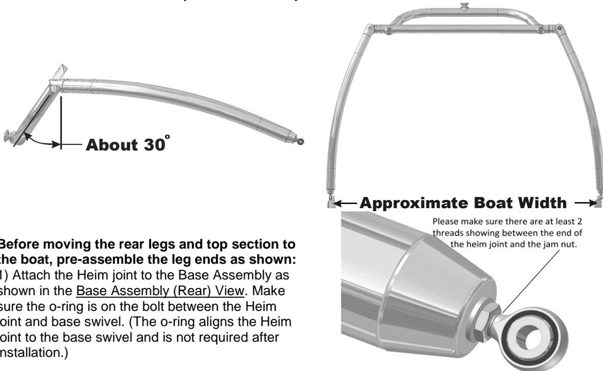
**Before moving the rear legs and top section to the boat, pre-assemble the leg ends as shown:**
