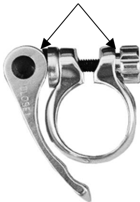
Quick release lubrication points
